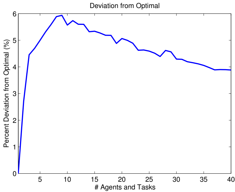
Figure 2-6: Diagonal slice of the CBAA performance graph representing the worst-cases of the values
